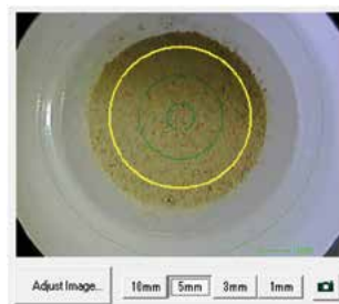
5 mm dia. Collimator Selected, Using Micro X-Cell
